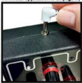
Plug the 3.5mm jack on the end of your Pin Wire Leads into the Lead Plug-In (located on the top edge of your P.E.S. Power Box XS).
