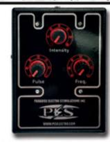
All three knobs should be turned completely to the left/counter-clockwise (as you look at the face of the box while holding it.)
